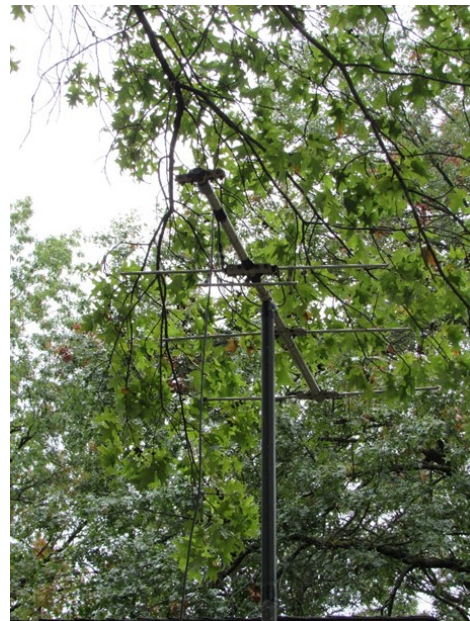
The modified 2-meter yagi, now with 3 elements instead of 4 elements.
